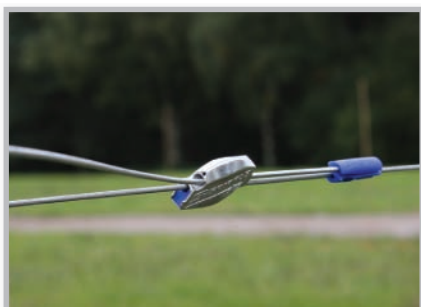
Join plain wire using Gripple Plus and a Twister
