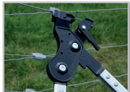
Tension plain wire with a Gripple tensioning tool
