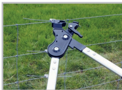
Tension field fence with a Gripple tensioning tool
